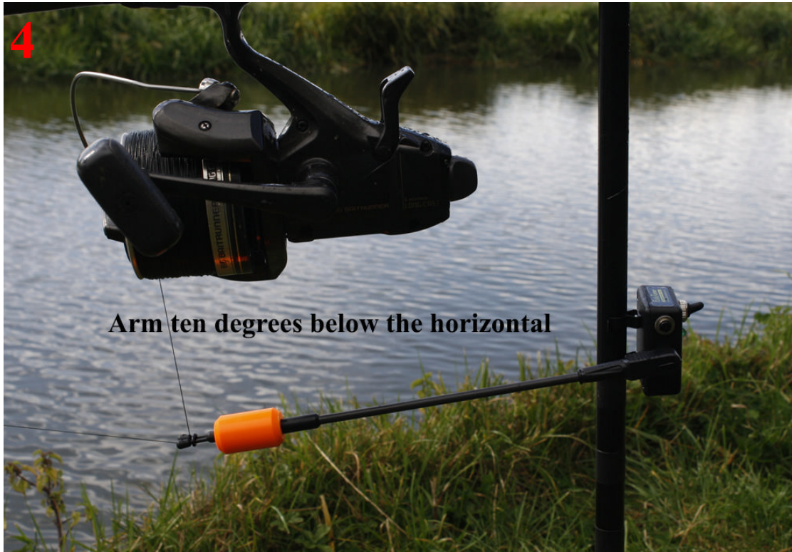
The arm here is ten degrees below horizontal which is the point that engages the audible buzzer (or ATTx/Auxiliary Buzzer) and LED
