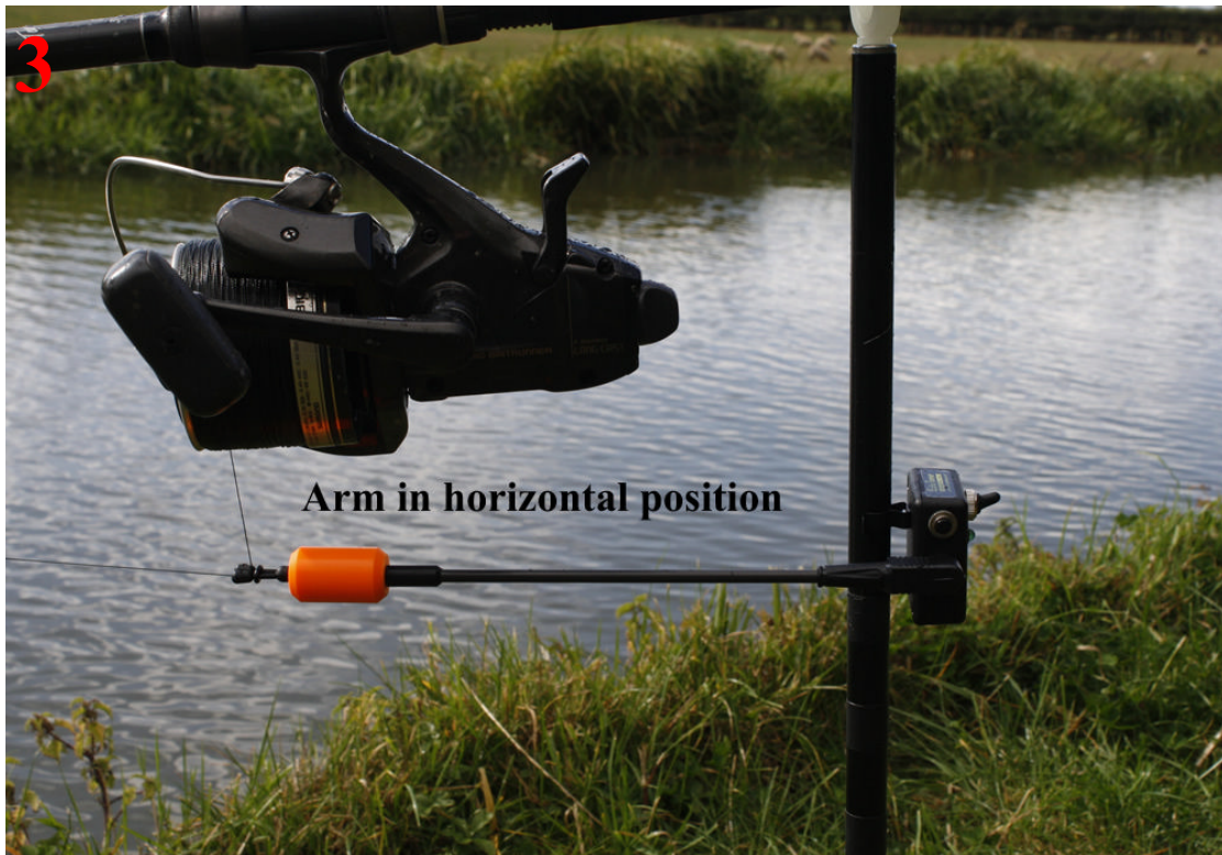
The arm here is in the horizontal position (alarm does not sound)
